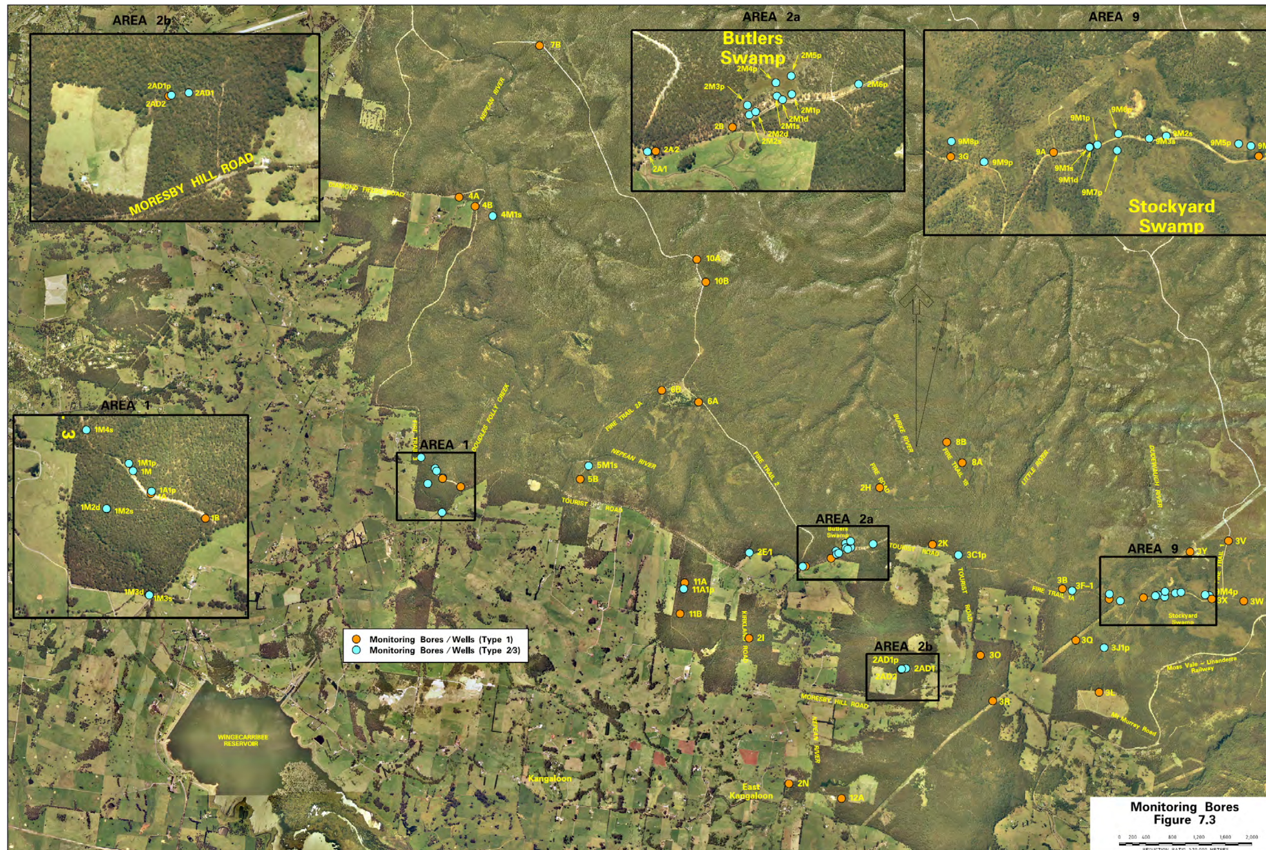
Figure 4.5 – Kangaloon Borefield – Current groundwater monitoring locations
