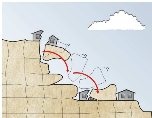
Figure 1 - Failure of an undercut block
